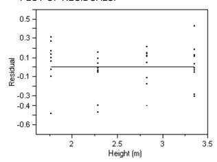
The plot of residuals does not suggest any major problems with the linear model. At each height, both positive and negative values may be observed and there is no obvious pattern to the residuals. The envelope, or outermost points, in the residual plot appears curved; however, if one covers the residual point in the upper right corner, the apparent curvature disappears. This suggests that there is no true pattern of curvature -- only an envelope that suggests curvature to the inexperienced eye.
